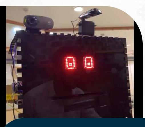
A Robotic lab assistant is a smart Robot that can guide the visitors throughout the lab, provide video surveillance security from unauthorized person, provide documentation of each project developed in lab, and enable efficient digital inventory management system.
