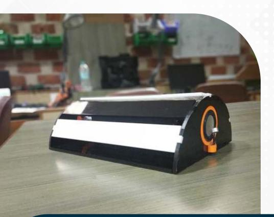
Description: The objective of this project to design low cost Sound Reactive Bluetooth Speakers. The audio/sound has been mapped to the neopixel LED's for making it react to the amplitude of sound connected via bluetooth.
