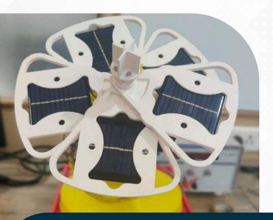
Description: This project aims to capture maximum intensity in minimum possible space (flower shape) and rotate whole set of solar panel in sun moving direction so that efficiency can maximize. It tracks sun movement and changes its face toward sun just like sunflower
